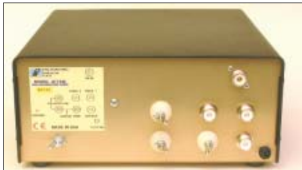
Real panel connections on the AT1KM (the AT1500CV is very similar).
